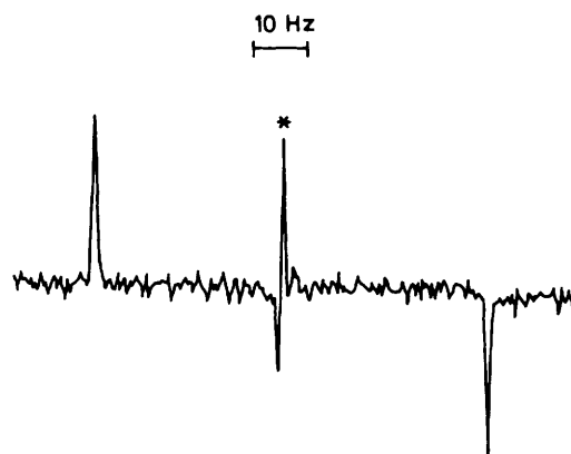
Figure 3. An example of observation of ^{15}\text{N} - ^1\text{H} coupling in a ^1\text{H} spectrum via multiple quantum n.m.r. Compound (10), ca. 20% solution in \text{CDCl}_3 , 5-mm sample tube, sweep width 600 Hz, 200 scans. A signal marked * is due to an incompletely suppressed signal from protons bonded to ^{14}\text{N}
